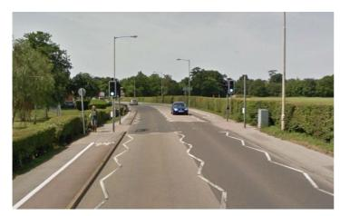
Toucan crossings are similar to puffin or pelican crossings but they are also designed to be used by cyclists. They consist of dropped kerbs, tactile paving, traffic signals to control flow and sometimes high friction surfacing on the approaches.
