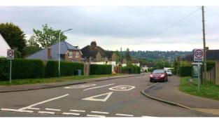
without additional measures due to the physical layout of the road, on-street parking etc. otherwise physical traffic calming measures will be needed to go along with the introduction of the change in the speed limit. This can include gateway treatments, speed humps, chicanes, road narrowing, and other measures to both physically and visually reinforce the reduced speed limit. It is worth noting that while residents may
