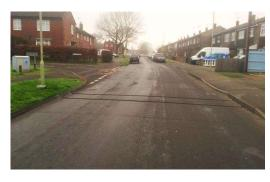
connected to a data logger that allows reports such as traffic volume, speed and vehicle classification to be generated. This type of count would generally be carried over a week-long period.
